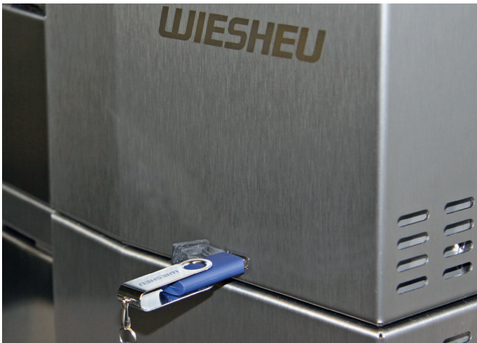
Programming of control unit via USB port
